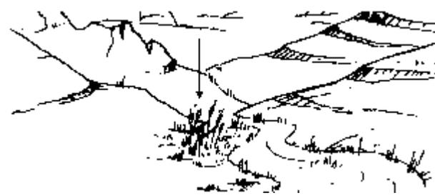
A V-box is constructed or a drum-well set in the wetland to contain water and to provide a draw-off point to lead to a tap or reservoir
